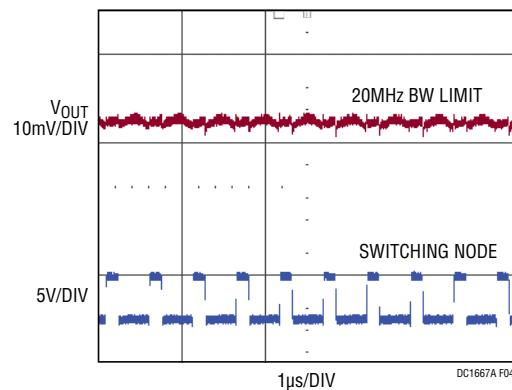
Figure 4. Measured Output Voltage Ripple at 5V Input,
