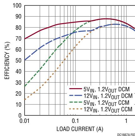
Figure 3. Measured Efficiency ( $V_{OUT} = 1.2V$ )
