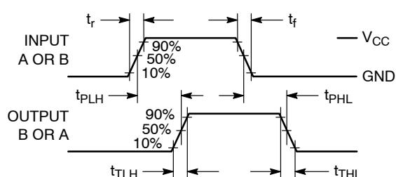
**Figure 3. Switching Waveform**
