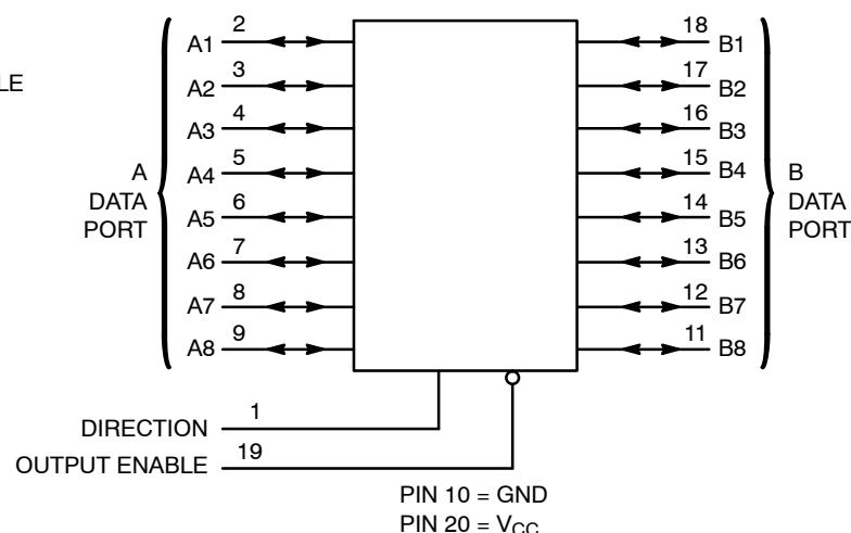
Figure 1. Pin Assignment
