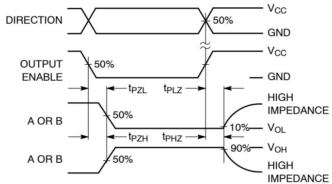
**Figure 4. Switching Waveform**
