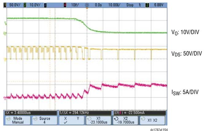
Figure 4. Short Circuit Waveforms with Frequency Foldback
