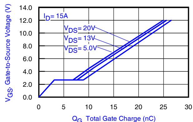
Fig 2. Typical Total Gate Charge vs Gate-to-Source Voltage
