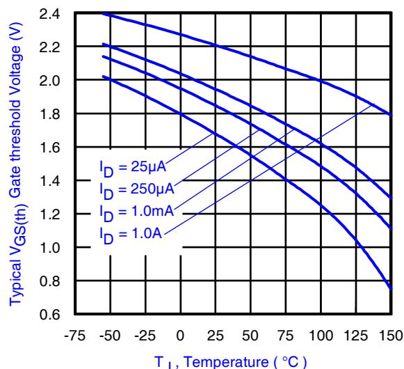
**Fig 13.** Typical Threshold Voltage vs. Junction Temperature
