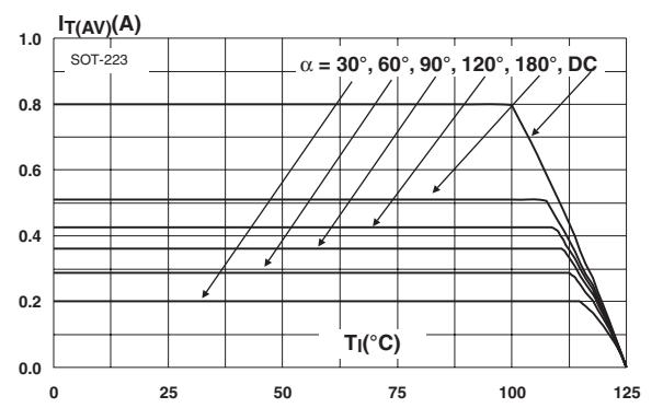
**Figure 4. Average and DC on-state current versus ambient temperature (free air convection)**
