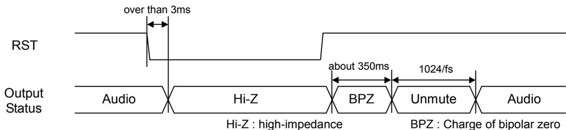
Figure 1. Reset Timing
