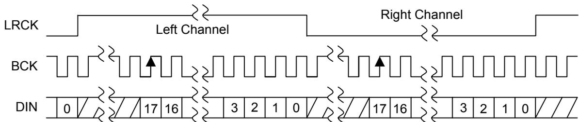
Figure 3.6. 18 bits LSB Justified Data Format
