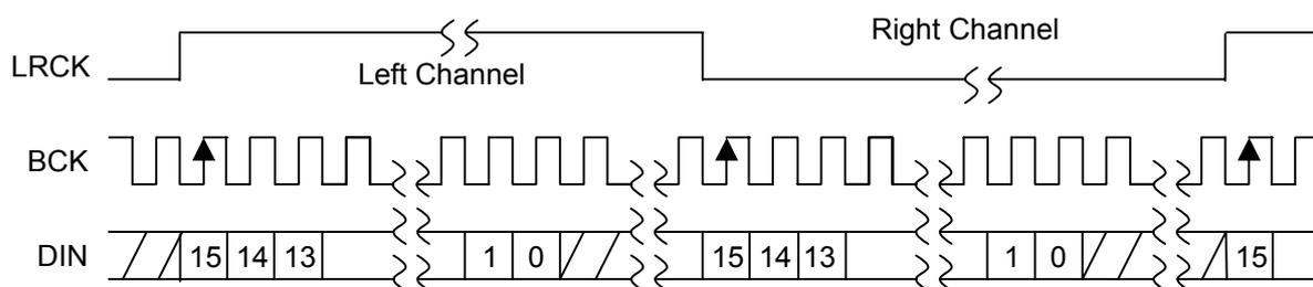
Figure 3.2. 16 bits MSB Justified Data Format
