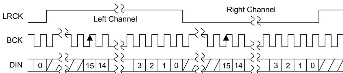
Figure 3.3. 16 bits LSB Justified Data Format
