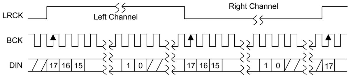
Figure 3.5. 18 bits MSB Justified Data Format
