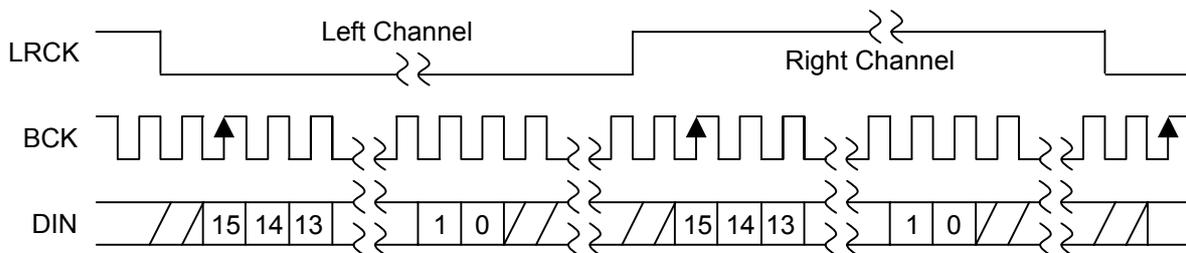
Figure 3.1. 16 bits I<sup>2</sup>S Data Format
