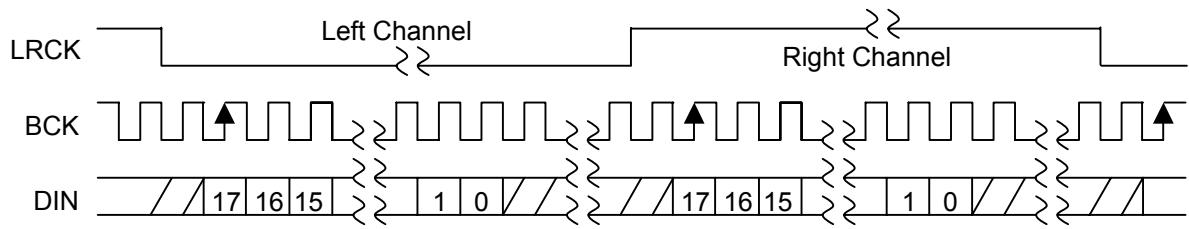
Figure 3.4. 18 bits I<sup>2</sup>S Data Format
