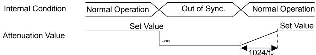
Figure 4. Out of Synchronization Operation
