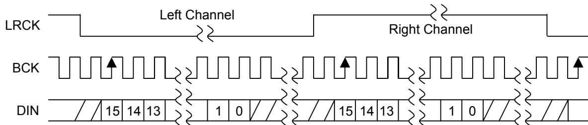
Figure 3.1. 16 bits I<sup>2</sup>S Data Format
