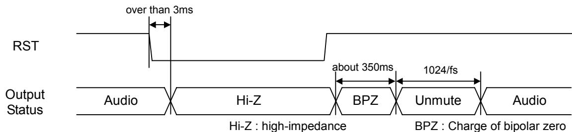
Figure 1. Reset Timing
