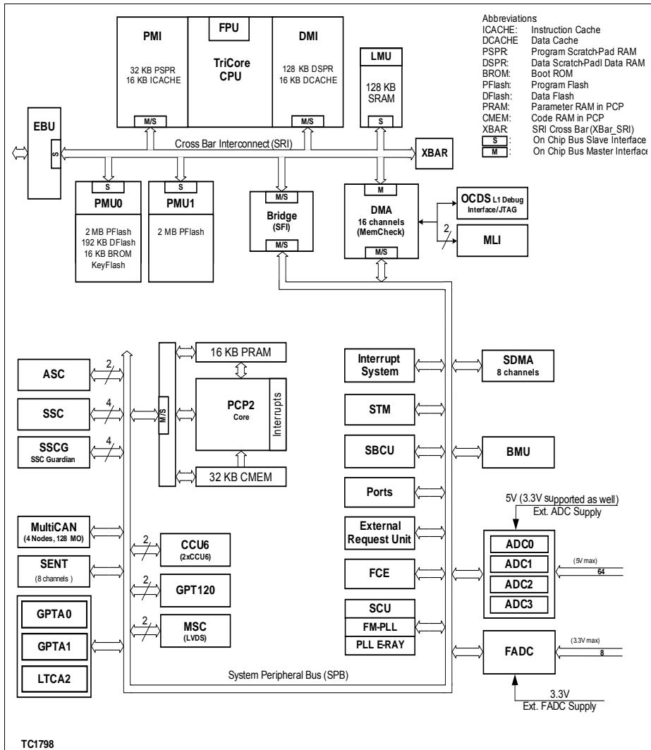
**Figure 3 Block Diagram**
