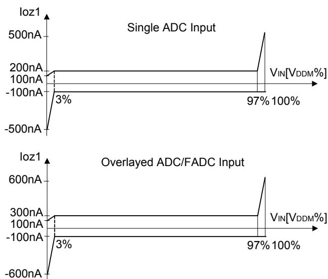
Figure 7 ADCx Analog Inputs Leakage
