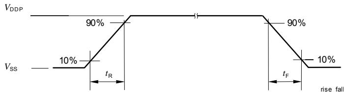
**Figure 9** Rise/Fall Time Parameters
