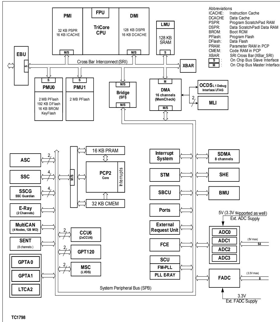
**Figure 1** Block Diagram
