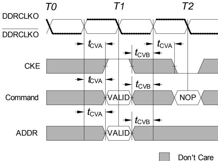
**Figure 30 DDR command and Address Timing**
