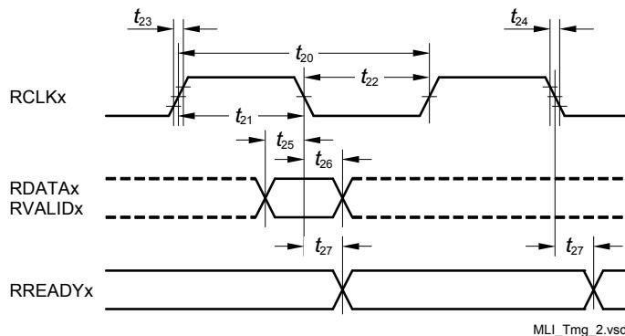
**Figure 19 MLI Interface Timing**
