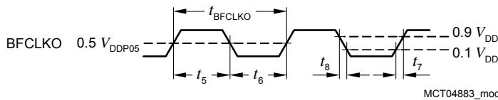
Figure 24 BFCLKO Output Clock Timing
