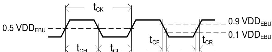
**Figure 29 Timing Waveform for DDR Clock Signals**
