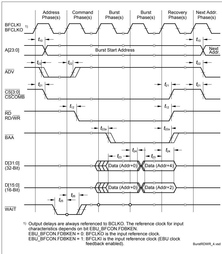
**Figure 27 EBU Burst Mode Read / Write Access Timing**
