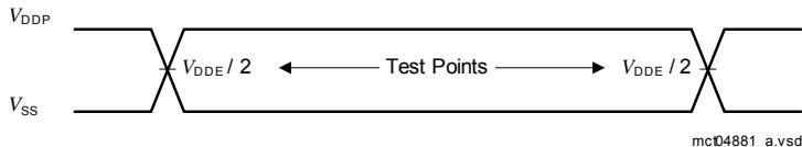
**Figure 10** Testing Waveform, Output Delay
