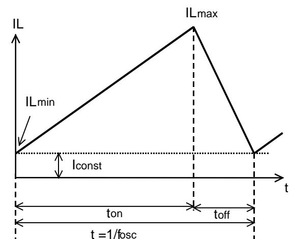
A PWM control type step-up DC/DC converter has two operation modes characterized by the continuity of inductor current: discontinuous current mode and continuous current mode.
