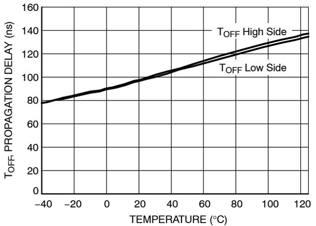
Figure 11. Turn OFF Propagation Delay vs. Temperature
