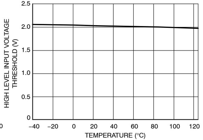
Figure 23. High Level Input Voltage Threshold vs. Temperature
