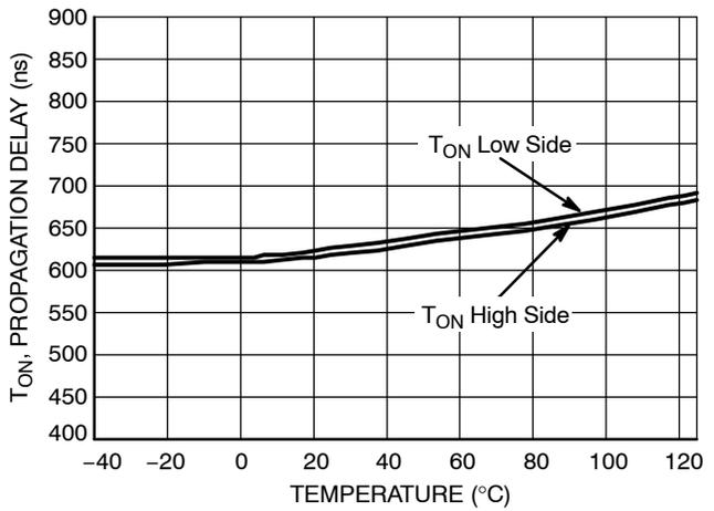
Figure 9. Turn ON Propagation Delay vs. Temperature
