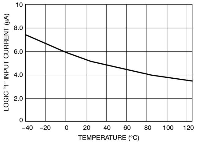
Figure 27. Logic "1" Input Current vs. Temperature
