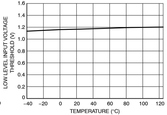
Figure 21. Low Level Input Voltage Threshold vs. Temperature
