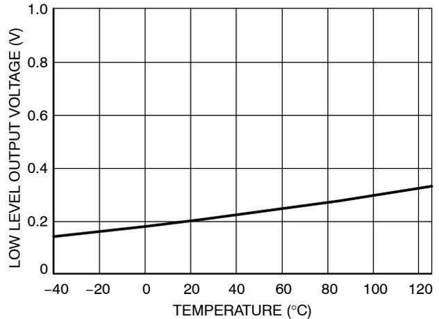
Figure 29. Low Level Output Voltage vs. Temperature
