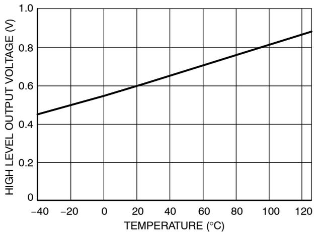
Figure 31. High Level Output Voltage vs. Temperature
