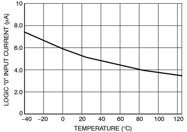
Figure 25. Logic "0" Input Current vs. Temperature
