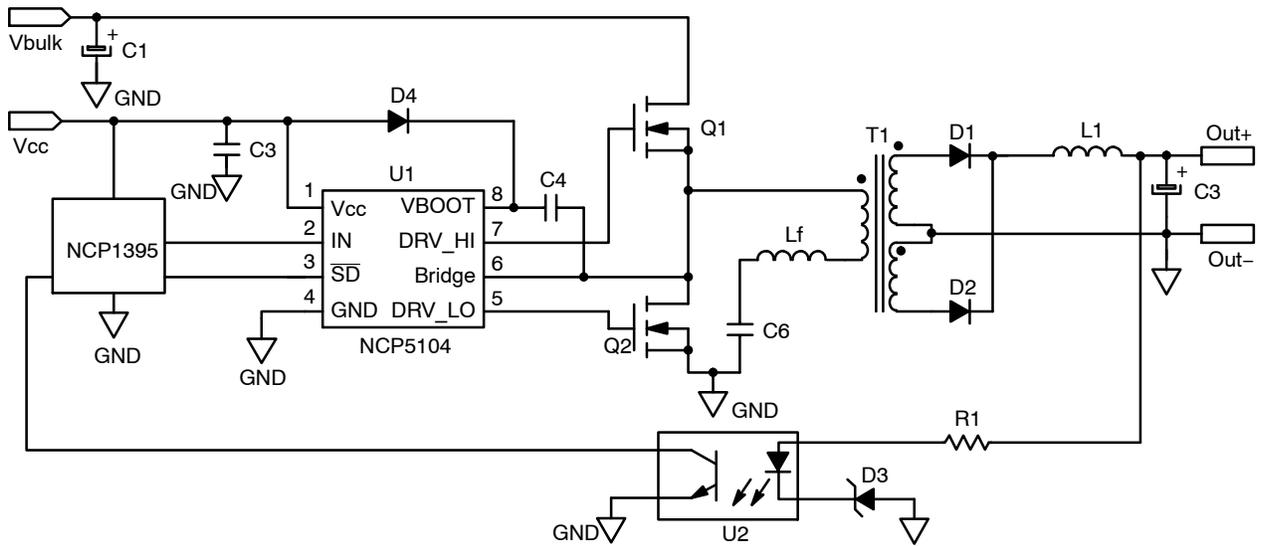
Figure 1. Typical Application Resonant Converter (LLC type)
