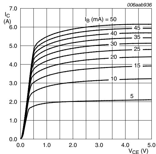
$T_{amb} = 25\text{ }^{\circ}\text{C}$ **Fig 6.** Collector current as a function of collector-emitter voltage; typical values
