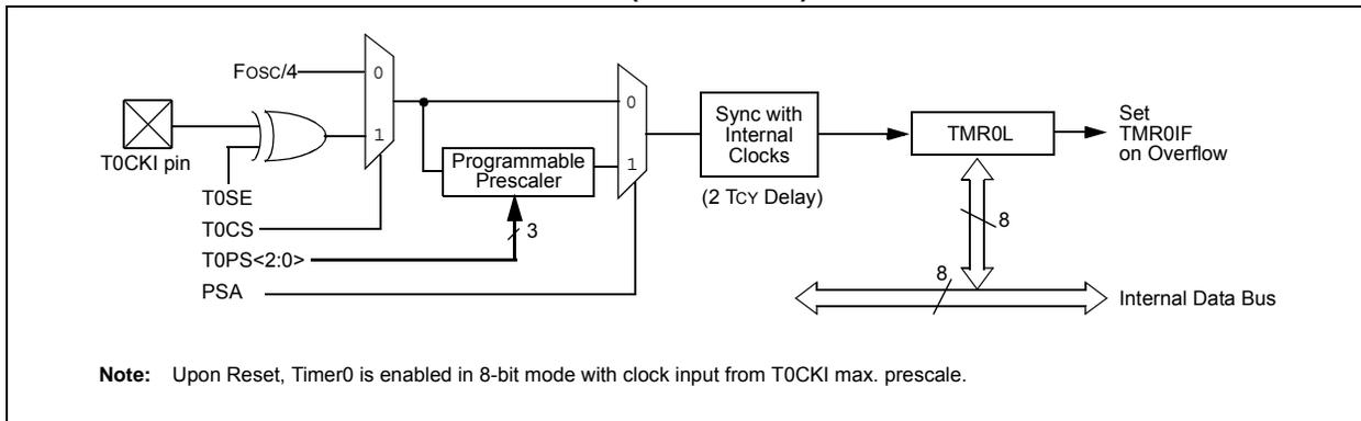
**FIGURE 11-2: TIMER0 BLOCK DIAGRAM (16-BIT MODE)**
