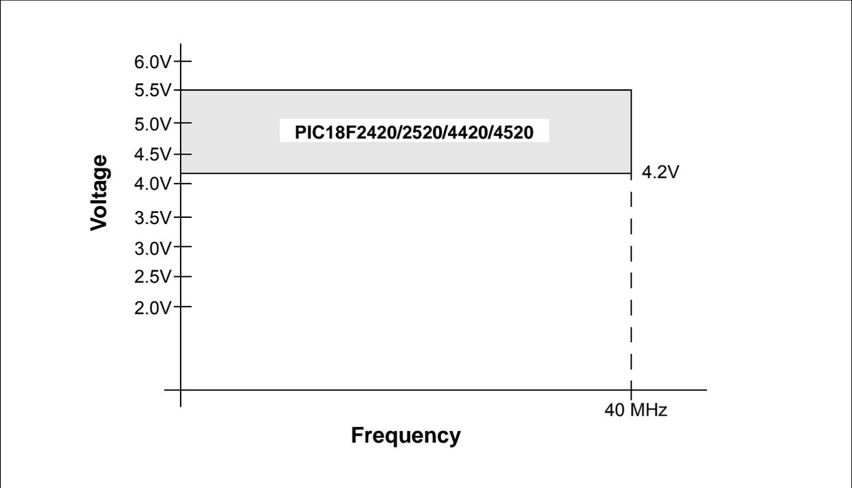
FIGURE 26-2: PIC18F2420/2520/4420/4520 VOLTAGE-FREQUENCY GRAPH (EXTENDED)
