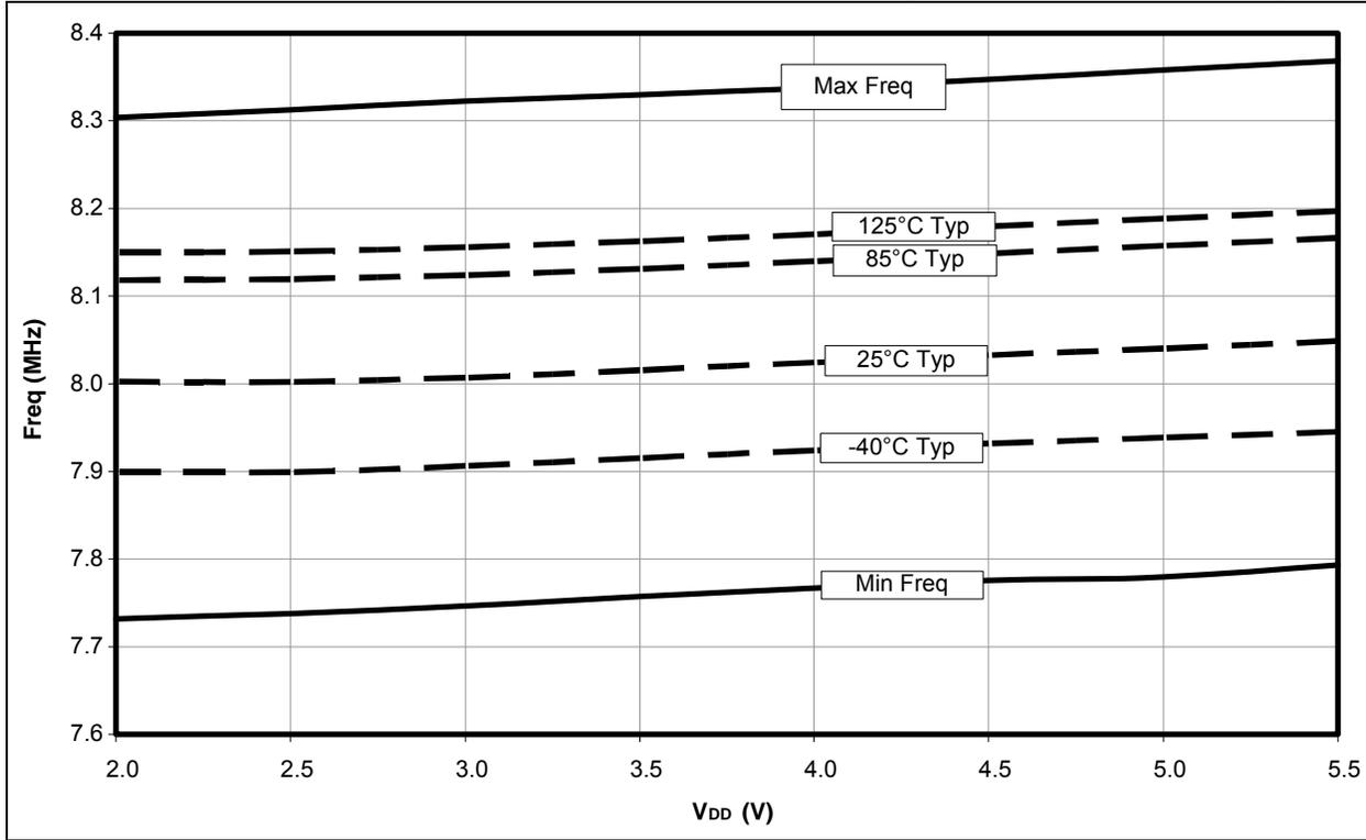
FIGURE 27-38: INTRC vs. V<sub>DD</sub> ACROSS TEMPERATURE (-40°C TO +125°C)
