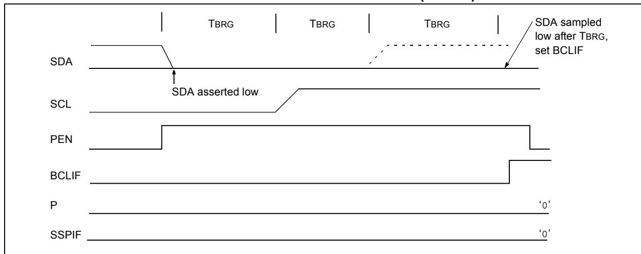
**FIGURE 17-32: BUS COLLISION DURING A STOP CONDITION (CASE 2)**
