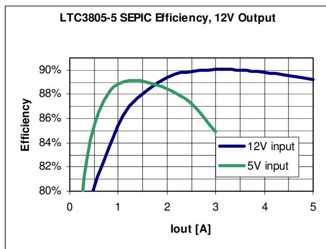
Figure 3. High efficiency of DC1576 allows the board to be used in thermally critical applications with outputs over 3A.
