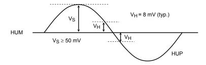
\*: The Hall amplifier can operate when V<sub>S</sub> is at least 50mVpp. However, to stabilize the time interval between zero-cross points of each phase signal, that is, the 60-electrical-degree interval, the amplitude should be as high as possible. (VS is recommended to be 200 mVpp or higher.)
