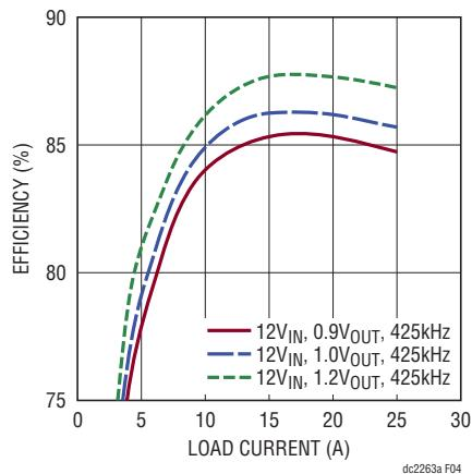
Figure 4. Typical Efficiency Curves DC2263A-A,  $f_{SW} = 425\text{kHz}$
