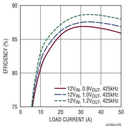
Figure 5. Typical Efficiency Curves DC2263A-B,  $f_{SW} = 425\text{kHz}$
