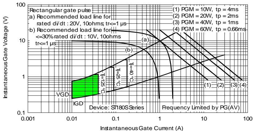
Fig. 9 - Gate Characteristics
