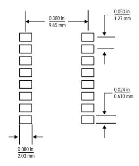
Figure 6. Footprint SOIC-16 (Case 475-01)
