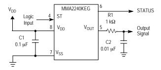
Figure 4. SOIC Accelerometer with Recommended Terminations
