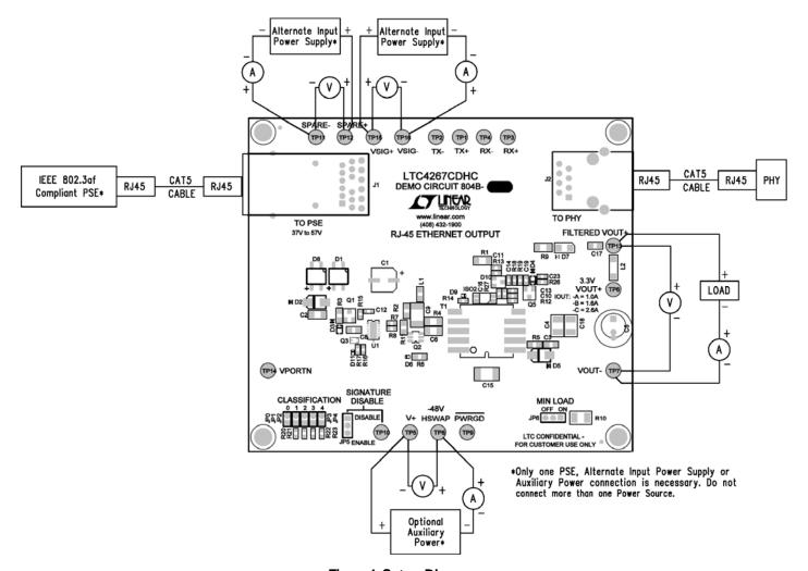
Figure 1. Setup Diagram
