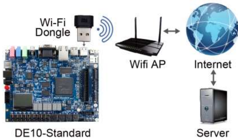
Figure 6-15 System diagram of USB Wi-Fi dongle
