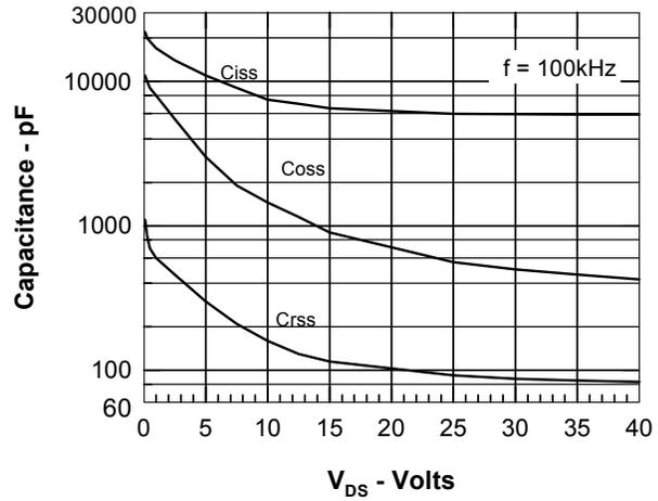
Fig.8 Capacitance Curves
