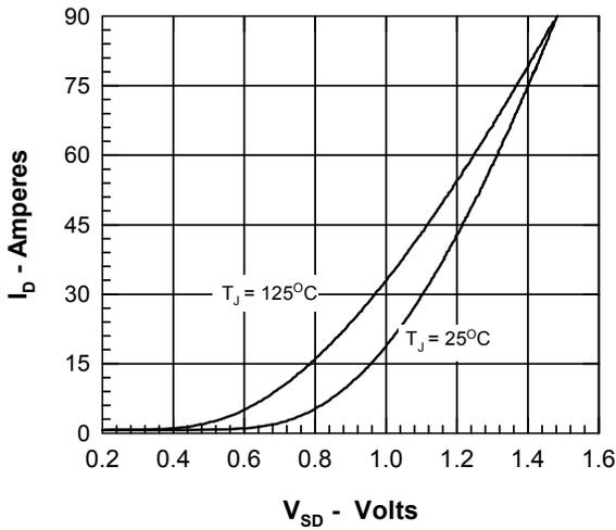
Fig.9 Drain Current vs Drain to Source Voltage
