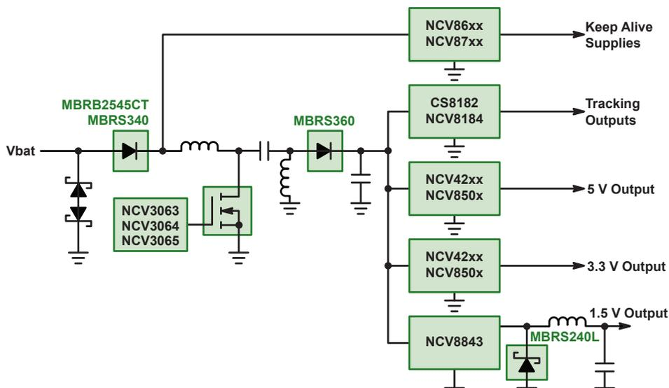
ON Semiconductor offers a wide selection of highly efficient power supply solutions that can handle harsh powertrain battery transients. The portfolio includes multi-topology controllers, such as NCV8871 and NCV3063, to provide regulated voltage greater than 5 V with a battery operating voltage between 4 V to 18 V; as well as buck regulators and controllers, like NCV8851 and NCV8843, to supply the high current, low voltage microcontroller cores.
