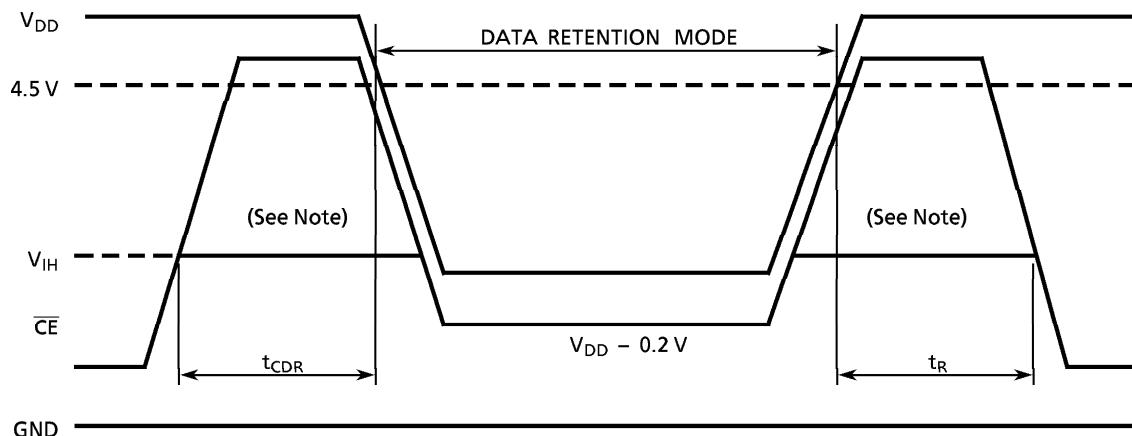
Note: When  $\overline{CE}$  is operating at the  $V_{IH}$  level (2.4 V), the standby current is given by  $I_{DDS1}$  during the transition of  $V_{DD}$  from 4.5 to 2.6 V.
