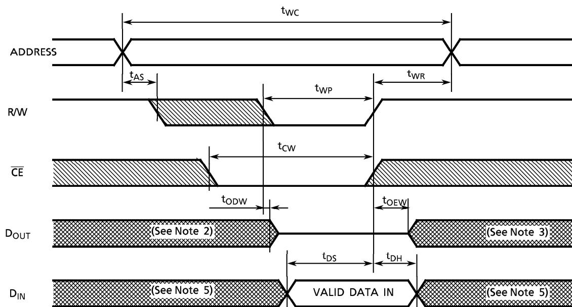
WRITE CYCLE 2 ( $\overline{CE}$  CONTROLLED) (See Note 4)
