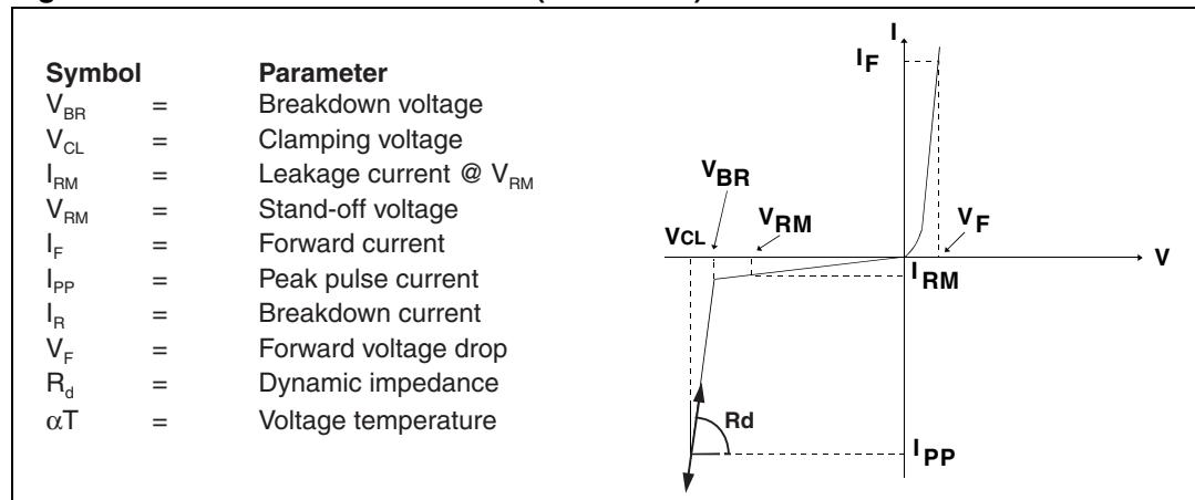
**Table 2. Electrical characteristics (values,  $T_{amb} = 25^\circ C$ )**
