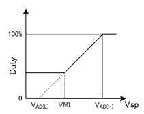
(PWM duty indicates the peak value of output because this circuit has a soft switching function.)
