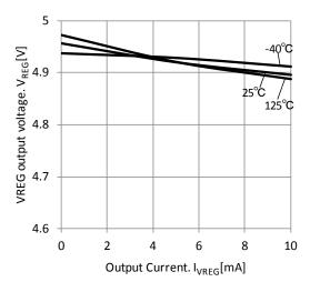
Fig.3 VREG pin voltage (VM=12V)
