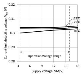
Fig.10 Current limit detecting voltage for RS pin
