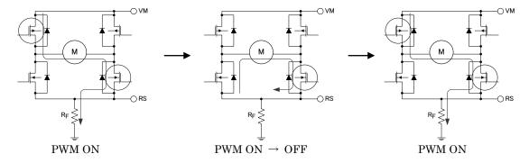
In switching phase, power transistor operates in below order.
