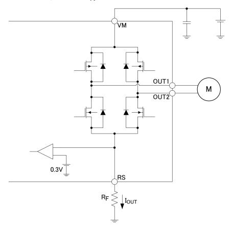
During the current limit operation, the operation mode is moved to PWM OFF state by turning off the upper output power transistor. The operation resumes at the next PWM ON timing.
