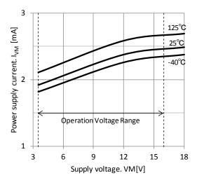
Fig.1 Power supply current
