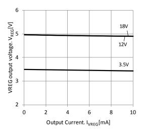
Fig.4 VREG pin voltage (Ta=25°C)
