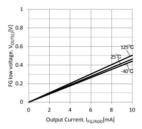
Fig.7 FG/RDO pin Output low voltage (VM=12V)
