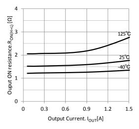
Fig.5 Output ON resistance (VM=12V)
