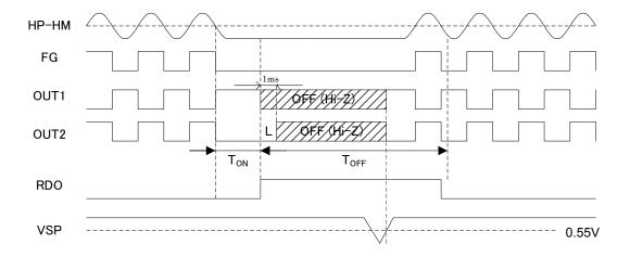
Because the voltage of VSP pin is detected through A/D circuit, the voltage of VSP pin should be kept at VAD(L) or less for VSP response time (TVSP) or more in order to clear the lock protection.
