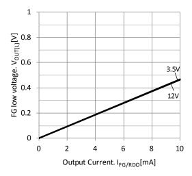
Fig.8 FG/RDO pin Output low voltage (Ta=25°C)
