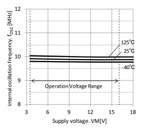
Fig.9 Internal oscillation frequency
