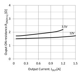
Fig.6 Output ON resistance (Ta=25°C)
