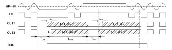
FG is outputted by the hall signal even while the lock protection is operating.
