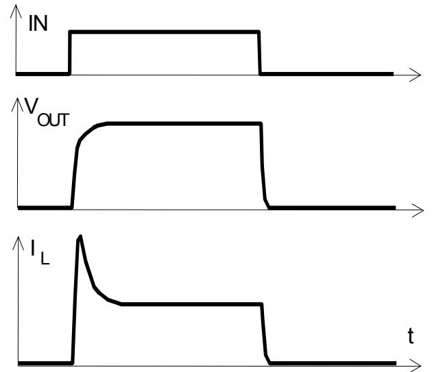
**Figure 2a:** Switching a resistive load,
