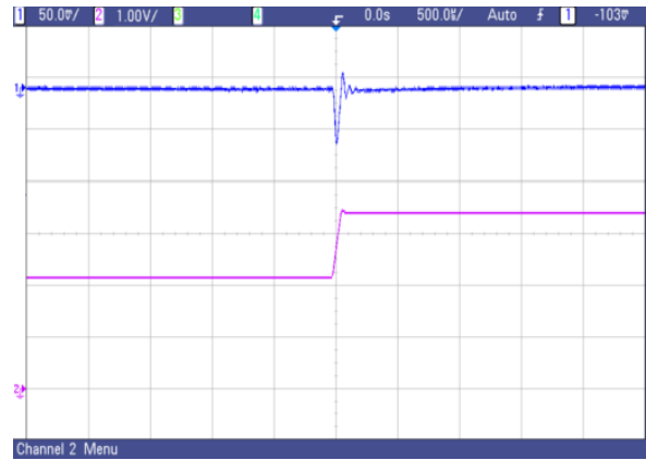
Fig. 23 AVO75-48S1V2 typical transient response to step increase in load from 50% to 75% of full load, room temperature, 48Vdc input
