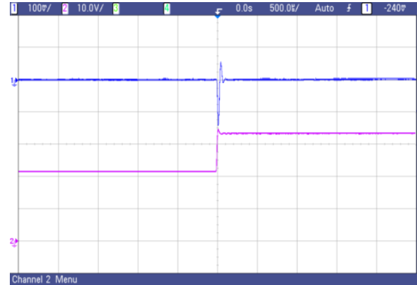
Fig. 37 AVO75-48S2V5 typical transient response to step increase in load from 50% to 75% of full load, room temperature, 48Vdc input ( \Delta I_o/\Delta t=1A/1\mu s )
