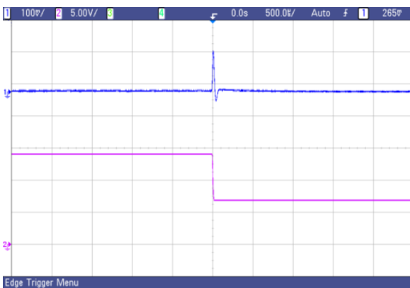
Fig. 44 AVO75-48S05 typical transient response to step decrease in load from 50% to 25% of full load, room temperature, 48Vdc input ( \Delta I_o/\Delta t=1A/1\mu s )
