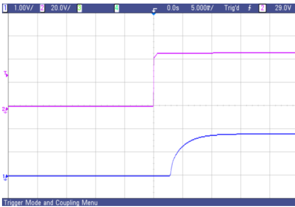
Fig. 61 AVO75-48S1V8 typical start-up from power on
