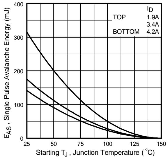
**Fig 15c.** Maximum Avalanche Energy Vs. Drain Current
