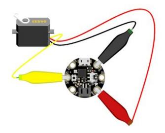
For **Gemma**, use jumper wire alligator clips to connect the ground wire to **GND**, the power wire to **VOUT**, and the signal wire to **A2**.
