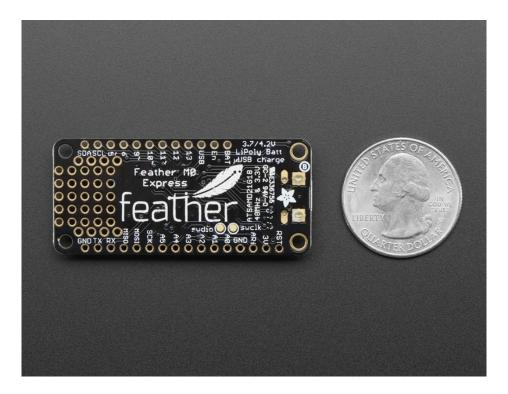
Comes fully assembled and tested, with a USB bootloader that lets you quickly use it with the Arduino IDE or for loading Circuit Python. We also toss in some header so you can solder it in and plug into a solderless breadboard.
