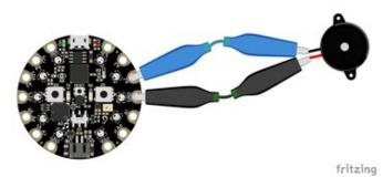
Use alligator clips to attach **A2** and any one of the **GND** to different legs of the piezo.
