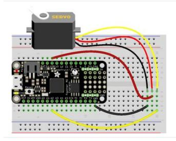
For boards like Feather M0 Express, ItsyBitsy M0 Express and Metro M0 Express, connect the ground wire to any GND, the power wire to USB or 5V, and the signal wire to A2.
