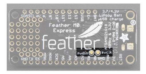
• **SWCLK & SWDIO** - These pads on the bottom are used to program the chip. They can also be connected to an SWD debugger.
