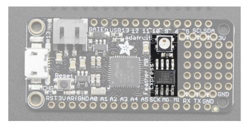
The **NeoPixel** is connected to pin #8 in Arduino, so just use our NeoPixel library (https://adafru.it/dhw) and set it up as a single-LED strand on pin 8. The NeoPixel is powered by the 3.3V power supply but that hasn't shown to make a big difference in brightness or color. The NeoPixel is also used by the bootloader to let you know if the device has enumerated correctly (green) or USB failure (red). In CircuitPython, the LED is used to indicate the runtime status.
