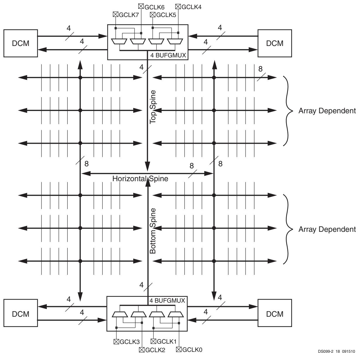
Figure 24: Spartan-3 FPGAs Clock Network (Top View)
