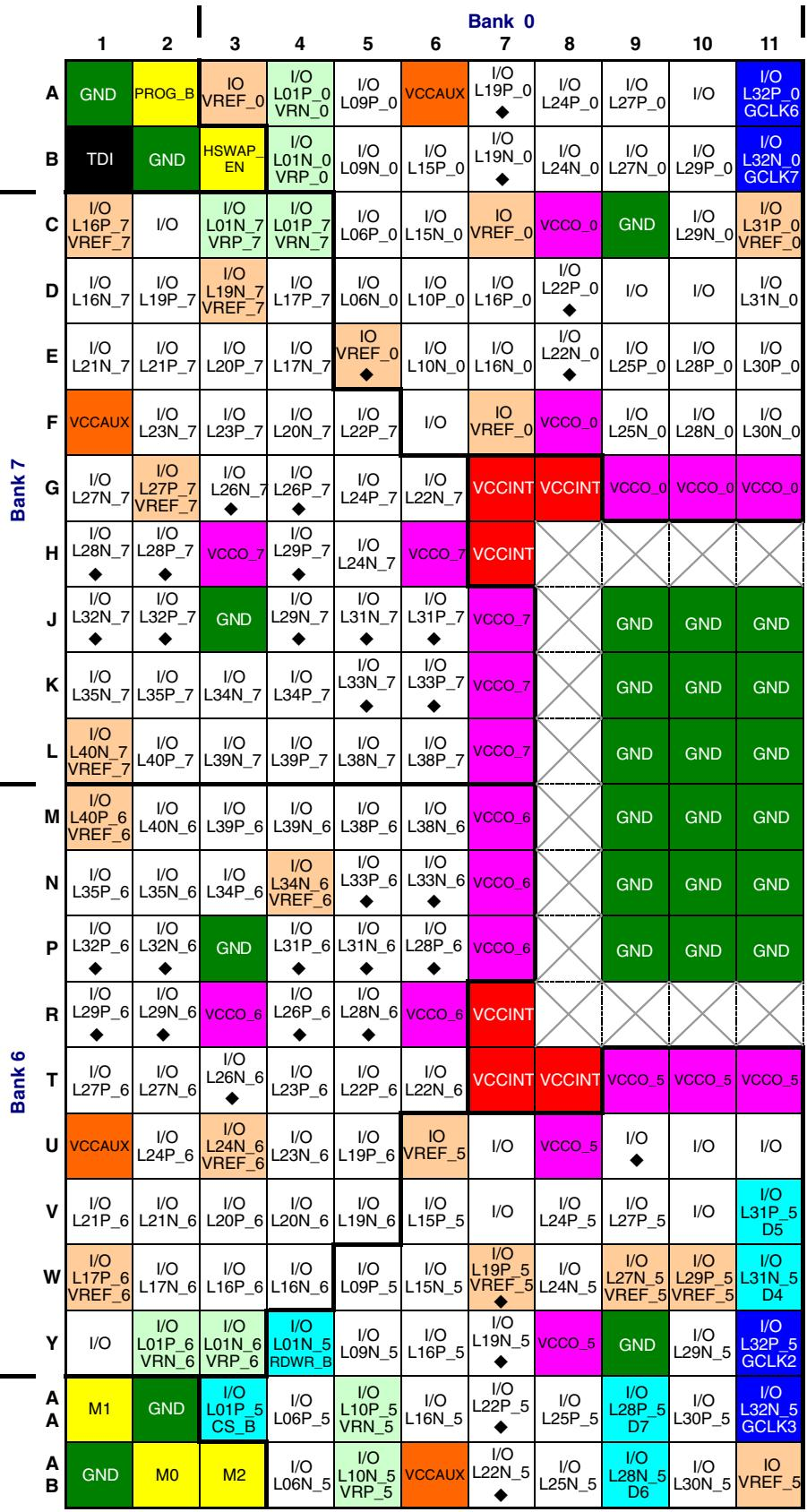
Figure 51: FG456 Package Footprint (Top View)
