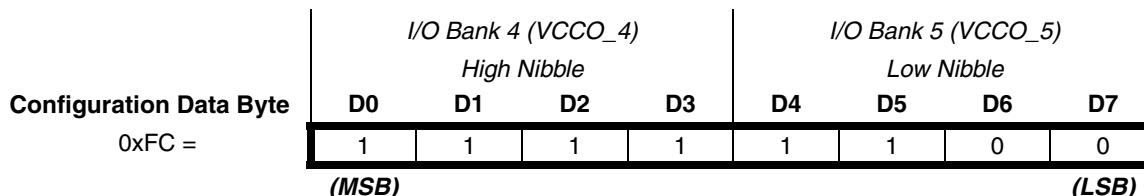
Figure 41: Configuration Data Byte Mapping to D0-D7 Bits
