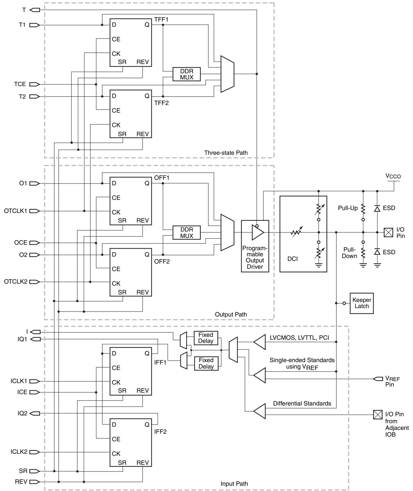
Note: All IOB signals originating from the FPGA's internal logic have an optional polarity inverter.
