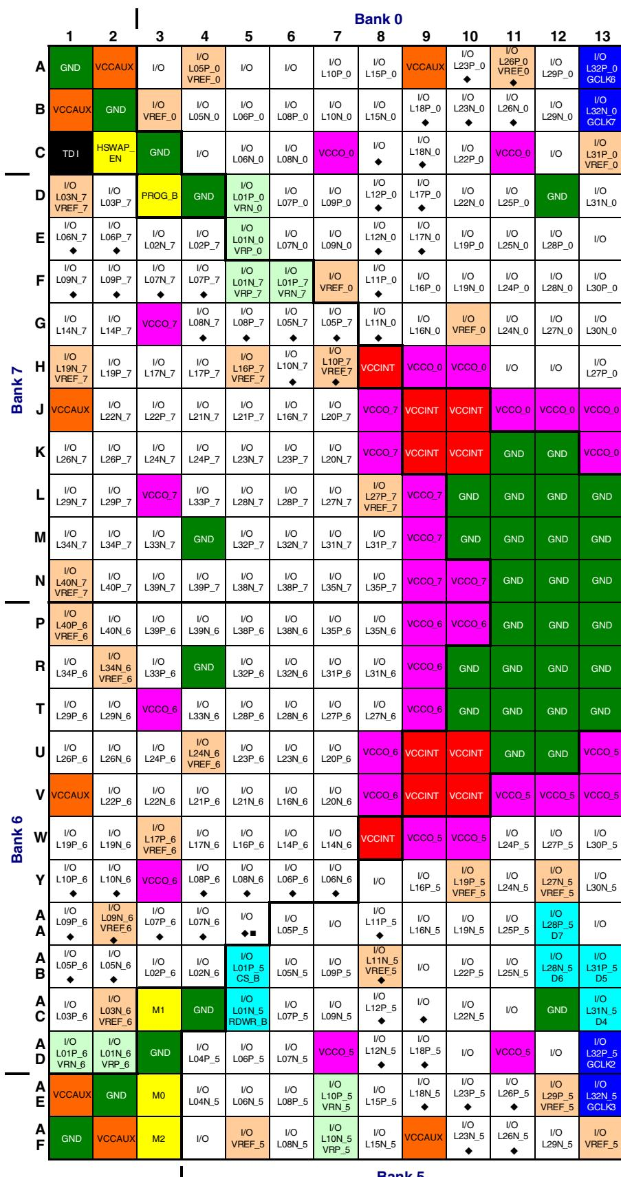
Figure 53: FG676 Package Footprint (Top View)
