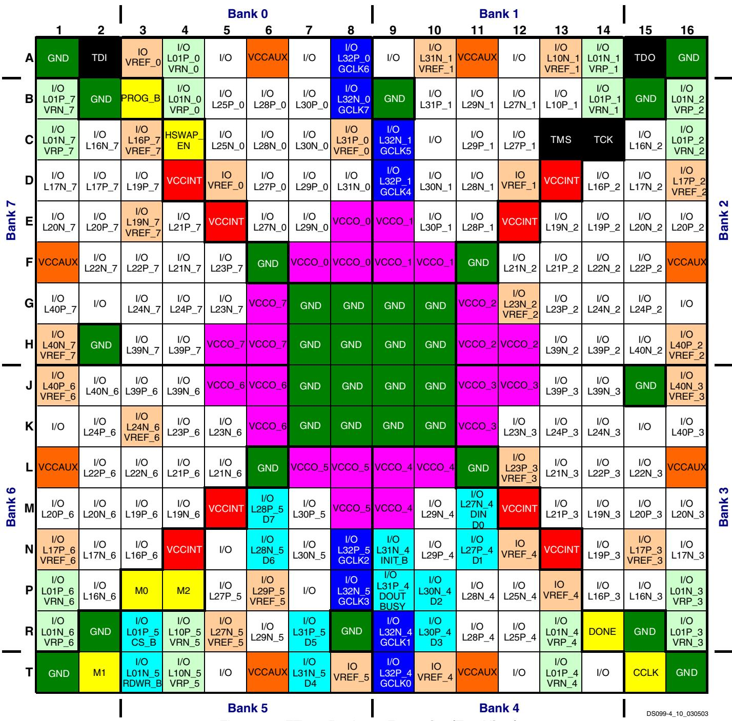
Figure 49: FT256 Package Footprint (Top View)
