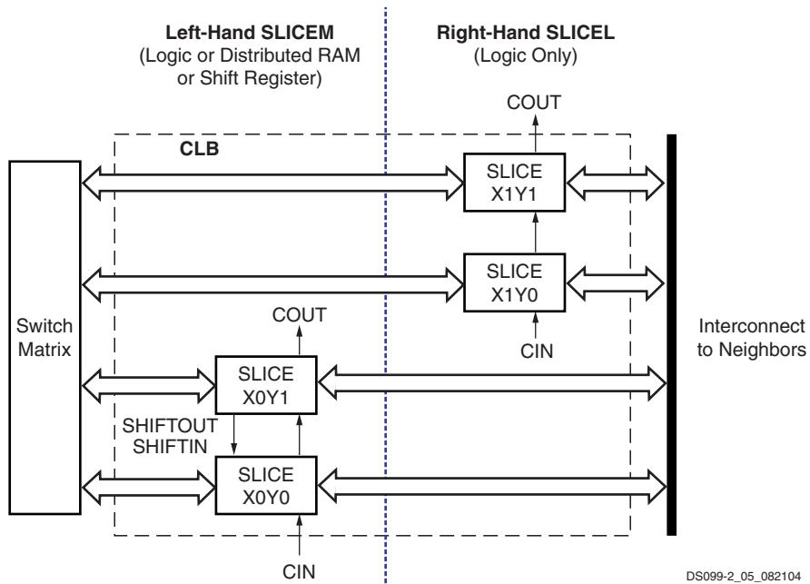
Figure 11: Arrangement of Slices within the CLB
