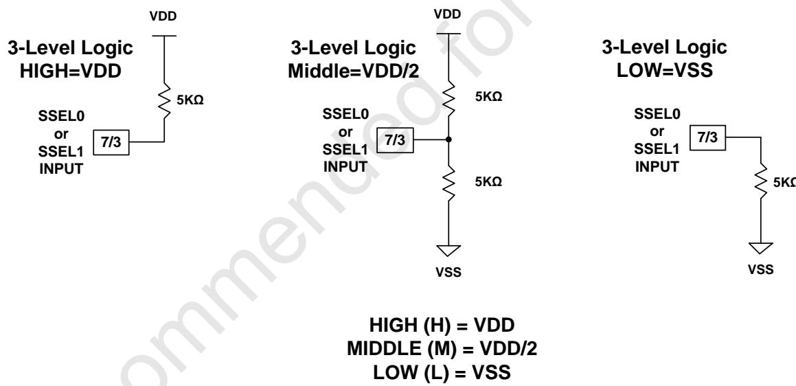
**Figure 3. FSEL0 and FSEL1 Spread % Selection Logic**
