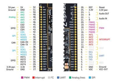
Figure 15: 1x26 pin header view
