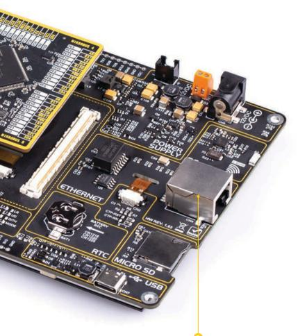
Figure 12: RJ-45 connector view
