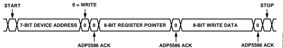
Figure 24. I 2 C Single Byte Write Sequence
