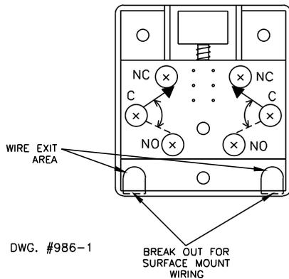
**Converting The HUB-M To Optional Latching Operation**
