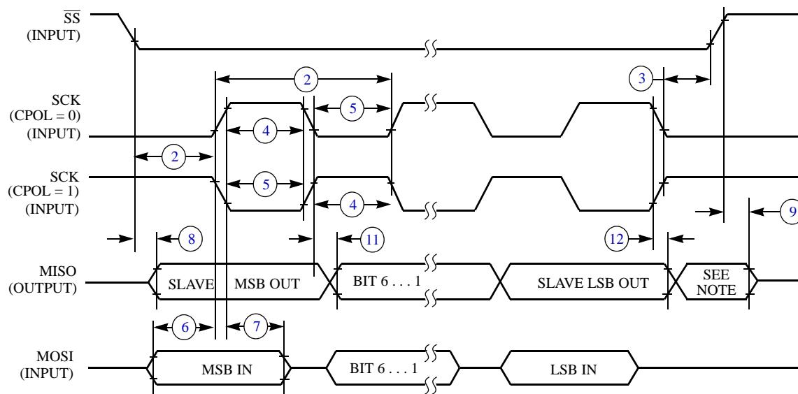
**Figure 17. SPI Slave Timing (CPHA = 0)**
