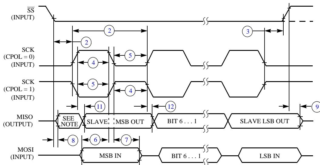
**Figure 18. SPI Slave Timing (CPHA = 1)**
