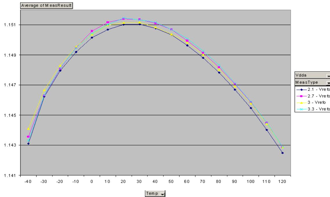
Figure 20. Typical VREF Output vs. V<sub>DD</sub>
