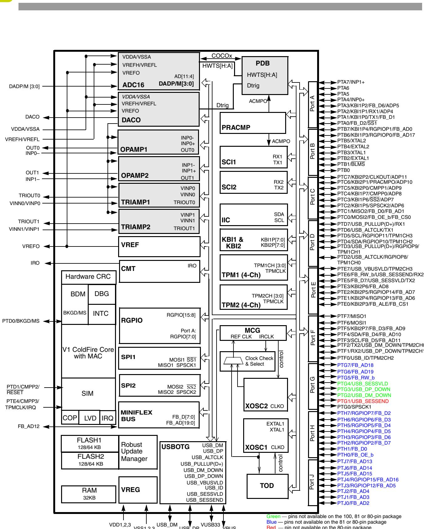
Figure 1. MCF51MM256 Series Block Diagram
