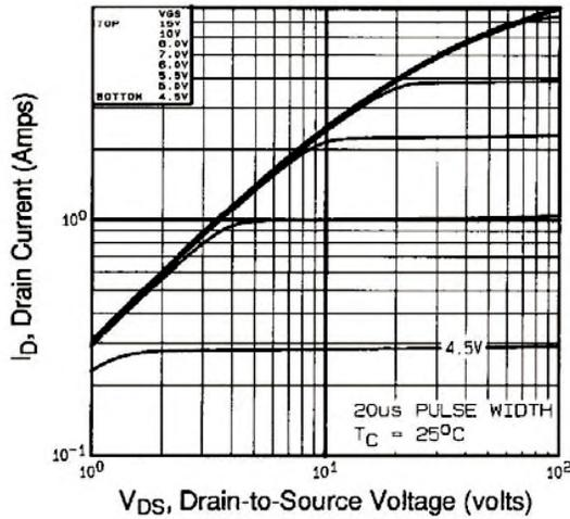
Fig. 1 - Typical Output Characteristics,  $T_C = 25\text{ }^\circ\text{C}$
