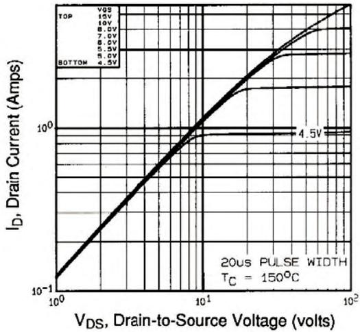
Fig. 2 - Typical Output Characteristics,  $T_C = 150\text{ }^\circ\text{C}$
