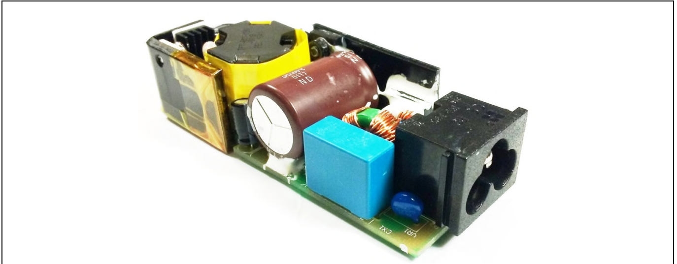
Figure 1 REF-45 W ADAPTER [PCBA dimensions L x W x H: 92 mm x 36mm x 22 mm]
