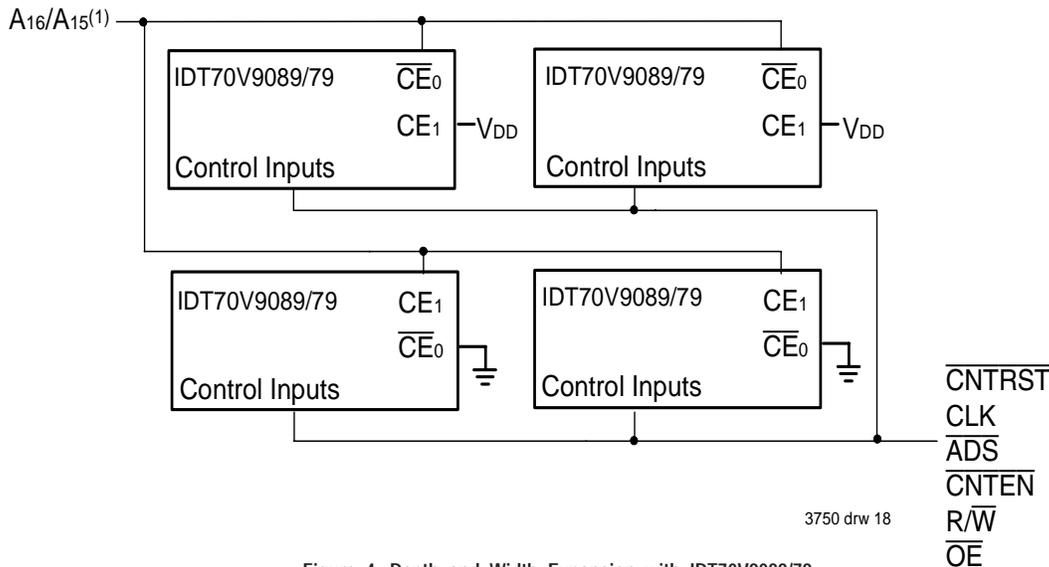
Figure 4. Depth and Width Expansion with IDT70V9089/79
