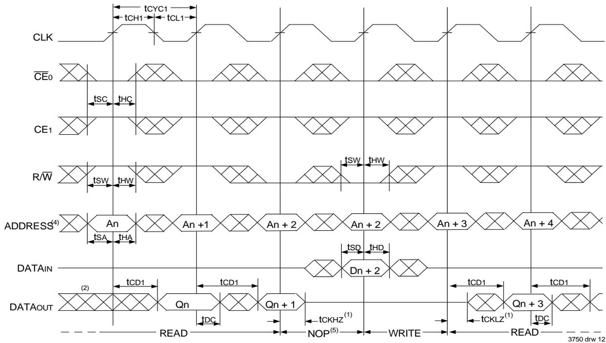
Timing Waveform of Flow-Through Read-to-Write-to-Read ( $\overline{OE}$  Controlled)<sup>(3)</sup>
