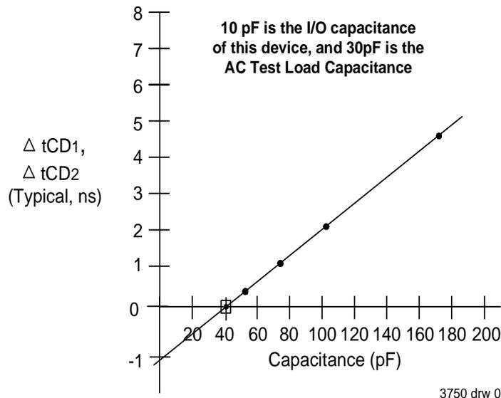
Figure 3. Typical Output Derating (Lumped Capacitive Load).
