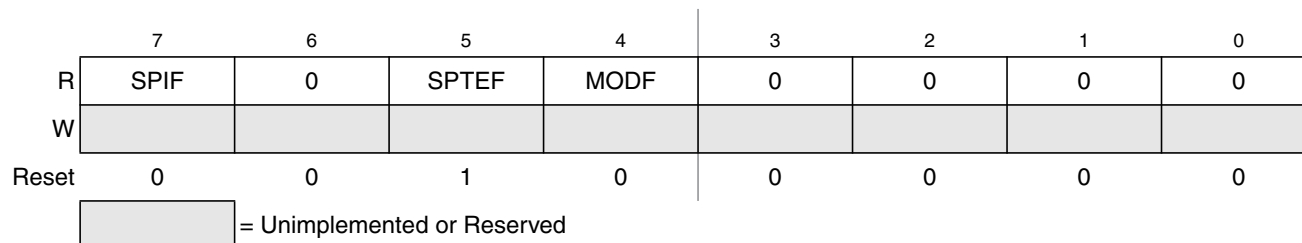
Figure 14-6. SPI Status Register (SPISR)
