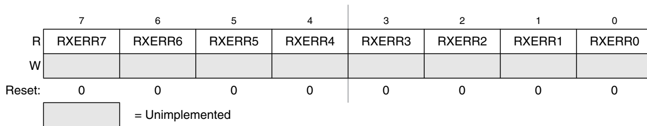
Figure 10-17. MSCAN Receive Error Counter (CANRXERR)
