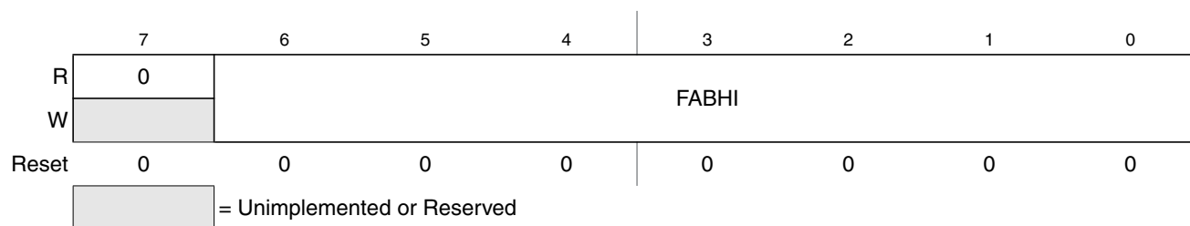
Figure 19-16. Flash Address High Register (FADDRHI)
