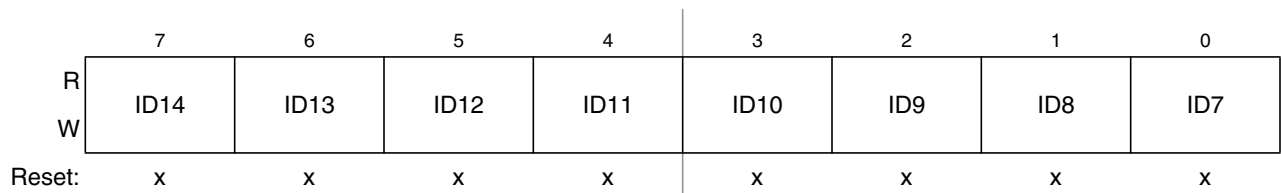
Figure 10-27. Identifier Register 2 (IDR2) — Extended Identifier Mapping
