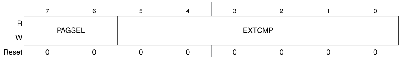
Figure 7-15. Debug Comparator A Extended Register (DBGCAx)
