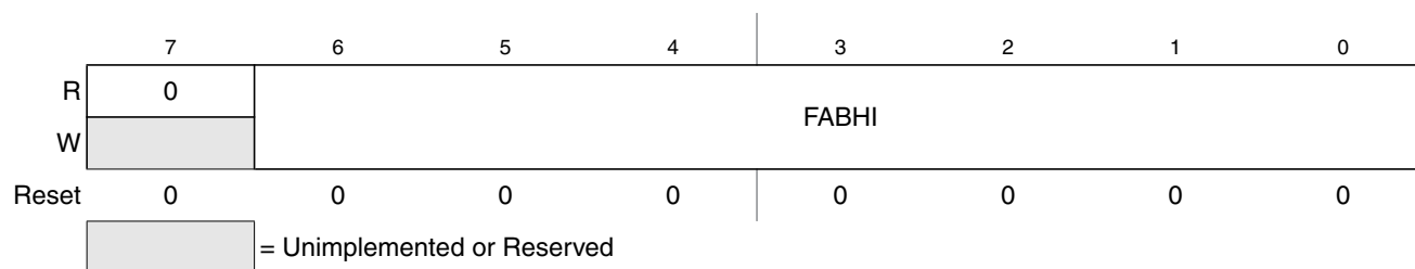
Figure 19-16. Flash Address High Register (FADDRHI)
