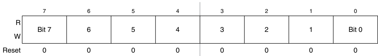
Figure 4-5. Data Direction Register B (DDRB)
