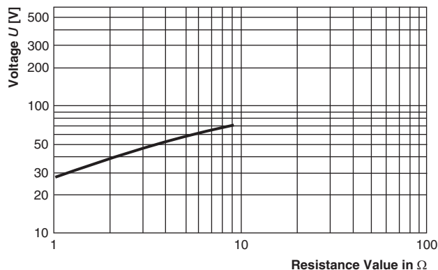
U_{max} . before Fusing and max. Pulse Voltage
