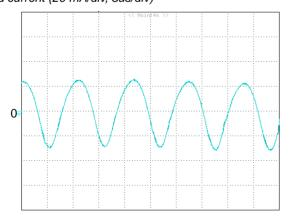
Figure 12: Output voltage ripple at nominal input voltage (Vin=48V) and rated load current (50 mV/div, 2us/div).Load capacitance: 1μF ceramic capacitor and 10μF tantalum capacitor. Bandwidth: 20 MHz. Scope measurements should be made using a BNC cable (length shorter than 20 inches). Position the load between 51 mm to 76 mm (2 inches to 3 inches) from the module
