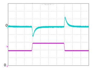
Figure 6: Output voltage response to step-change in load current (50%-75%-50% of lo, max; di/dt = 0.1A/μs; Vin is 24ν). Load cap: 10μF tantalum capacitor and 1μF ceramic capacitor. Top Trace: Vout (0.5V/div, 500us/div), Bottom Trace:lout (5A/div). Scope measurement should be made using a BNC cable (length shorter than 20 inches). Position the load between 51 mm to 76 mm (2 inches to 3 inches) from the module
