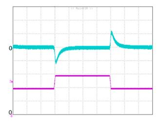
Figure 7: Output voltage response to step-change in load current (50%-75%-50% of lo, max; di/dt = 0.1A/µs; Vin is 48v). Load cap: 10µF tantalum capacitor and 1µF ceramic capacitor. Top Trace: Vout (0.5V/div, 500us/div), Bottom Trace: lout (5A/div). Scope measurement should be made using a BNC cable (length shorter than 20 inches). Position the load between 51 mm to 76 mm (2 inches to 3 inches) from the module
