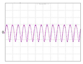
Figure 9: Input Terminal Ripple Current, i<sub>c</sub>, at full rated output current and nominal input voltage (Vin=48V) with 12µH source impedance and 33µF electrolytic capacitor (1A/div, 5us/div)
