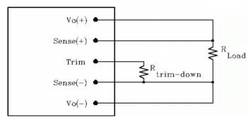
Figure 16: Circuit configuration for trim-down (decrease output voltage)
