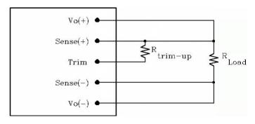
Figure 17: Circuit configuration for trim-up (increase output voltage)
