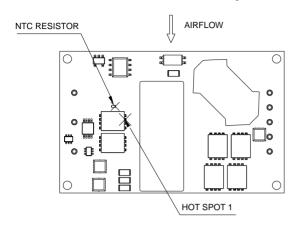
**Figure 19:** Temperature measurement location.\* The allowed maximum hot spot1 temperature is defined at 120  $^{\circ}$
