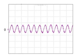
**Figure 10:** Input reflected ripple current, i<sub>s</sub>, through a 12μH source inductor at nominal input voltage (Vin=48V) and rated load current (20 mA/div, 5us/div)
