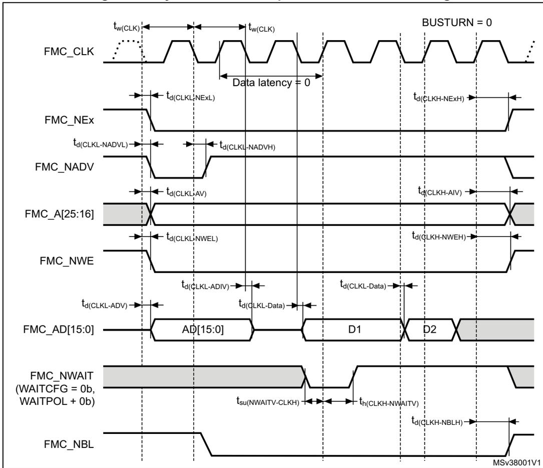
Table 100. Synchronous multiplexed PSRAM write timings<sup>(1)(2)</sup>
