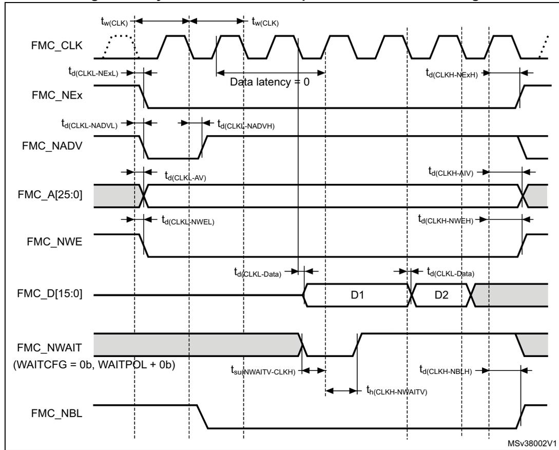
**Table 102. Synchronous non-multiplexed PSRAM write timings<sup>(1)(2)</sup>**
