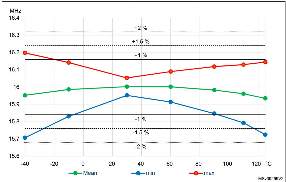
Multi-speed internal (MSI) RC oscillator
