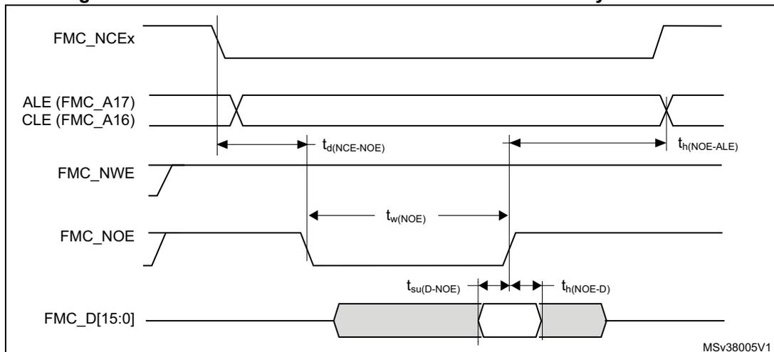
Figure 49. NAND controller waveforms for common memory write access
