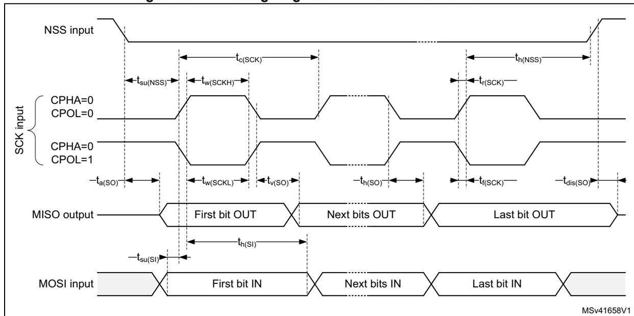
Figure 30. SPI timing diagram - slave mode and CPHA = 1
