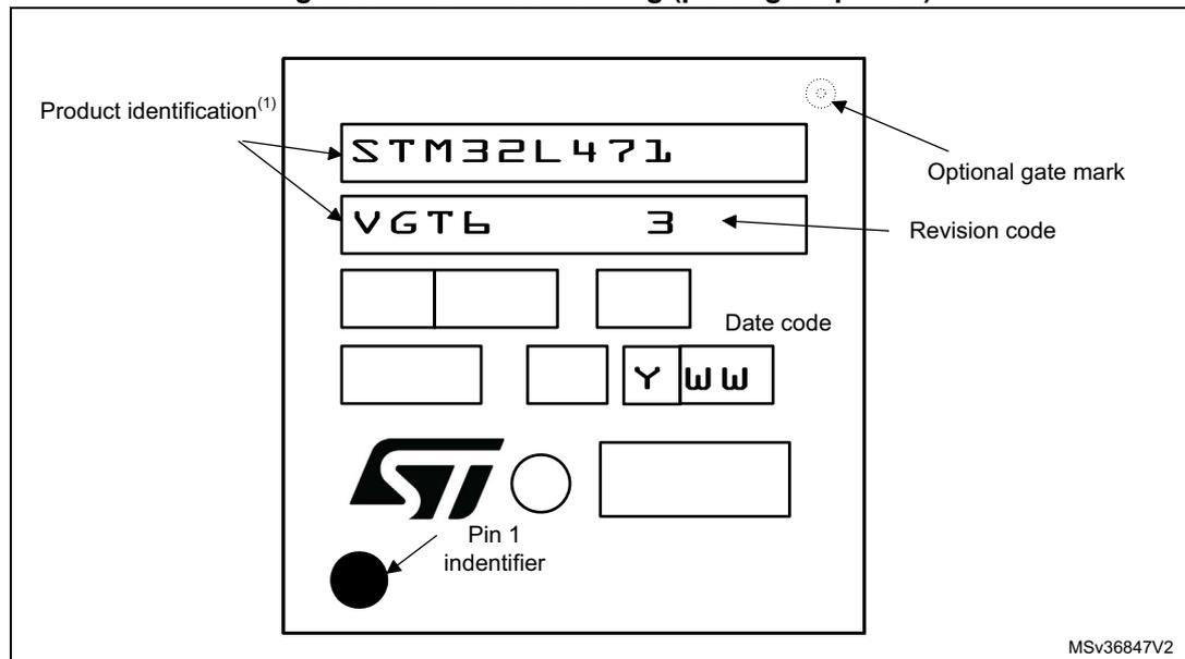
1. Parts marked as ES or E or accompanied by an Engineering Sample notification letter are not yet qualified and therefore not approved for use in production. ST is not responsible for any consequences resulting from such use. In no event will ST be liable for the customer using any of these engineering samples in production. ST's Quality department must be contacted prior to any decision to use these engineering samples to run a qualification activity.
