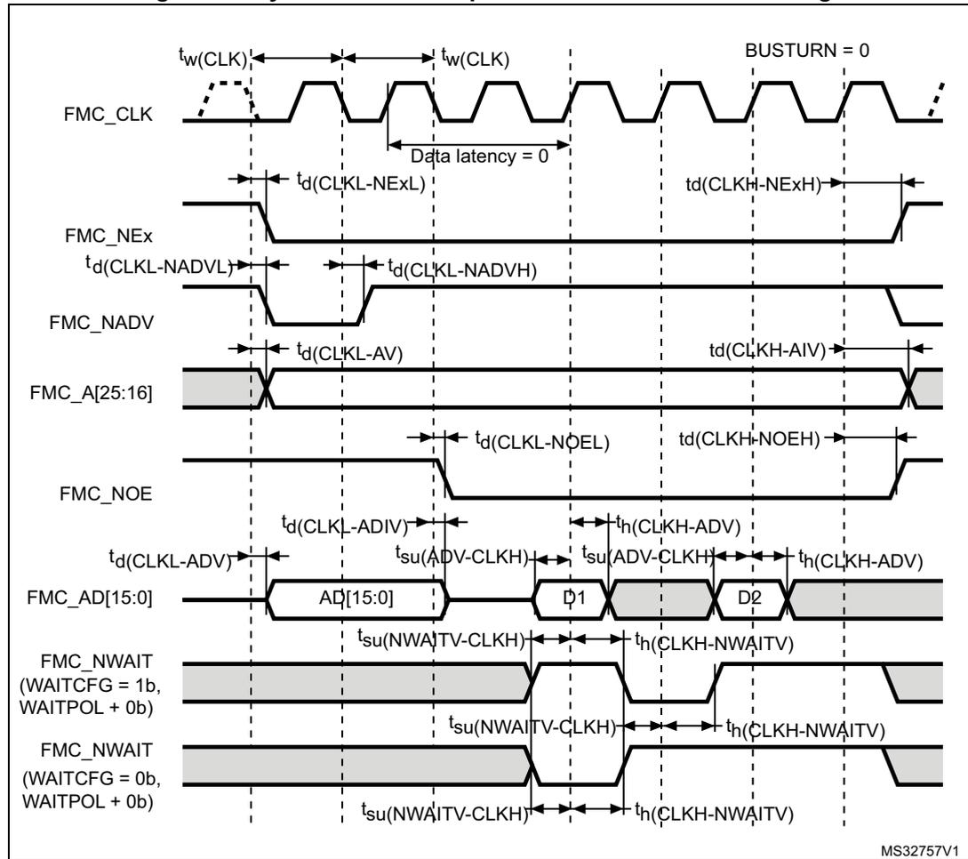
Table 99. Synchronous multiplexed NOR/PSRAM read timings<sup>(1)(2)</sup>
