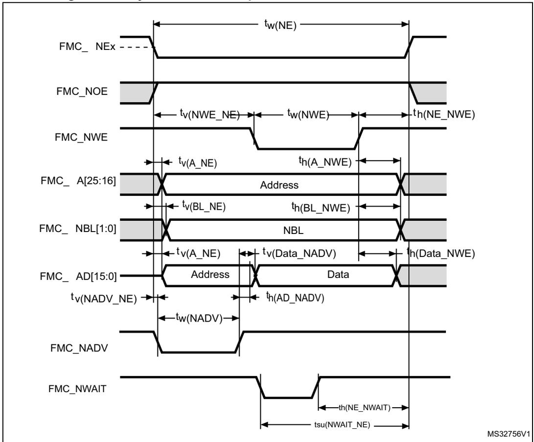
**Table 97. Asynchronous multiplexed PSRAM/NOR write timings<sup>(1)(2)</sup>**
