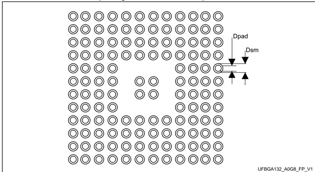
**Table 110. UFBGA132 recommended PCB design rules (0.5 mm pitch BGA)**
