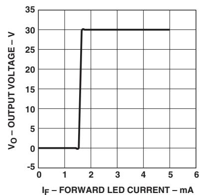
**Figure 15.** Transfer Characteristics.
