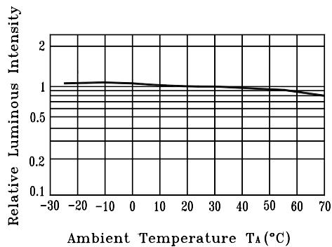
Fig.5 Luminous Intensity vs.
