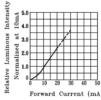
Fig.4 Relative Luminous Intensity
