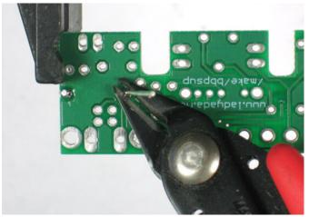
Now use yoru diagonal cutters to clip the long leads just above the solder joint.
