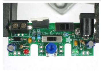
Next we will solder in the 2-pin terminal jack. This lets us connect up wires to power the board from a battery or similar.
